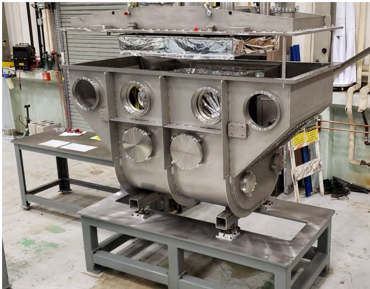
Figure 2.65. Vacuum vessel at ANL.
