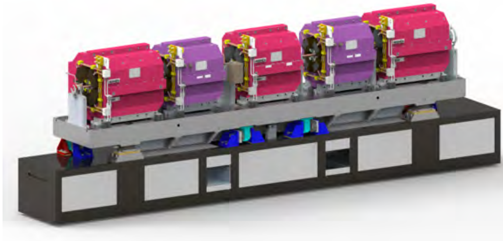
Figure 2.39. Preliminary FODO module assembly consists of (bottom to top) epoxy grout, concrete/steel plinth, cast iron support girder, individual magnets and vacuum system.
