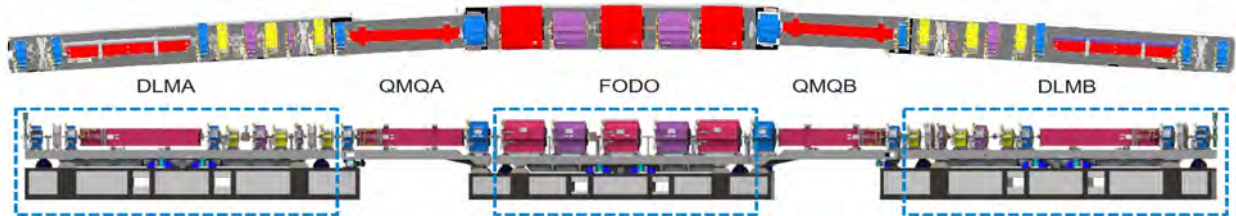
Figure 2.38. Plan and elevation views of the APS Upgrade lattice. The different magnet groups include two DLM modules, a FODO module, and two quadrupole / L-bend dipole / quadrupole (QM Q ) bridges. The DLM and FODO structures are supported from concrete plinths grouted to the floor, with QM Q modules supported by the ends of the plinths.
